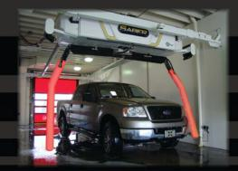
Auto-Resetting Breakaway Arms reset automatically in case of accidental vehicle strikes, maximizing uptime
