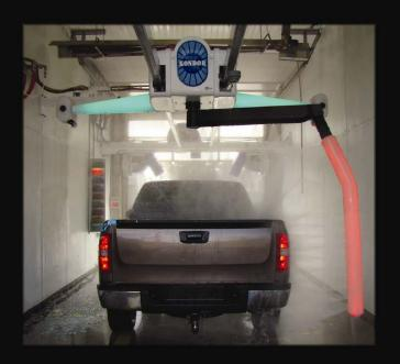
What's more, every Kondor® is built to impress. The narrow overhead rails form an 'inverted runway' that helps drivers get in position. The compact carriage head helps users feel safer, and eases diagnostic and service procedures from just two ladder positions. The Auto-Resetting Breakaway Arm resets itself without intervention. A stainless steel carriage frame is available based on your preference.
